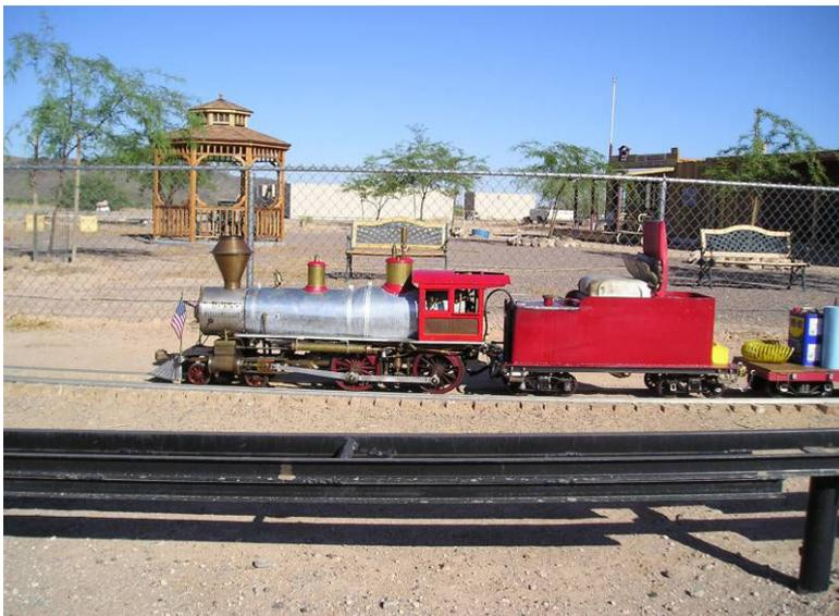
that choice of materials is less important than the quality and method of construction and care in operation. This particular 'American' has a steel boiler with silver soldered copper tubes. I am surprised that differential expansion does not cause problems, but I guess you just trade one set of potential problems for another. The boiler was originally hydro'd at 300 PSI (two years ago), and runs at around 100 PSI.
