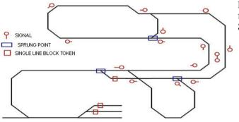
Left: Alan's diagram for Minimum Signalling
