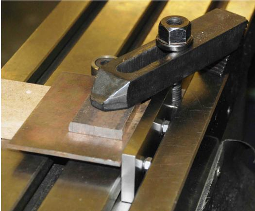
the table to locate the workpiece and a stop used to constrain the last of the so-called six degrees of freedom. The table T-slots can also be used to locate the workpiece. Other workholding devices including vices, vee blocks, angle plates, rotary tables, dividing head and tailstock can be fitted with tenons that fit snugly into the T-slots to facilitate accurate location and relocation following removal.
