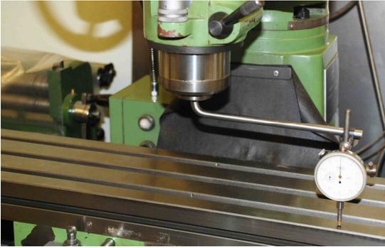
*Discussing the alignment of the vertical spindle of a milling machine, Mike showed how a plunger type dial gauge and L-formed bar is used to sweep from one side of the table to the other. Careful adjustment of the head brings the dial gauge readings the same each side and sets its axis vertical.*
