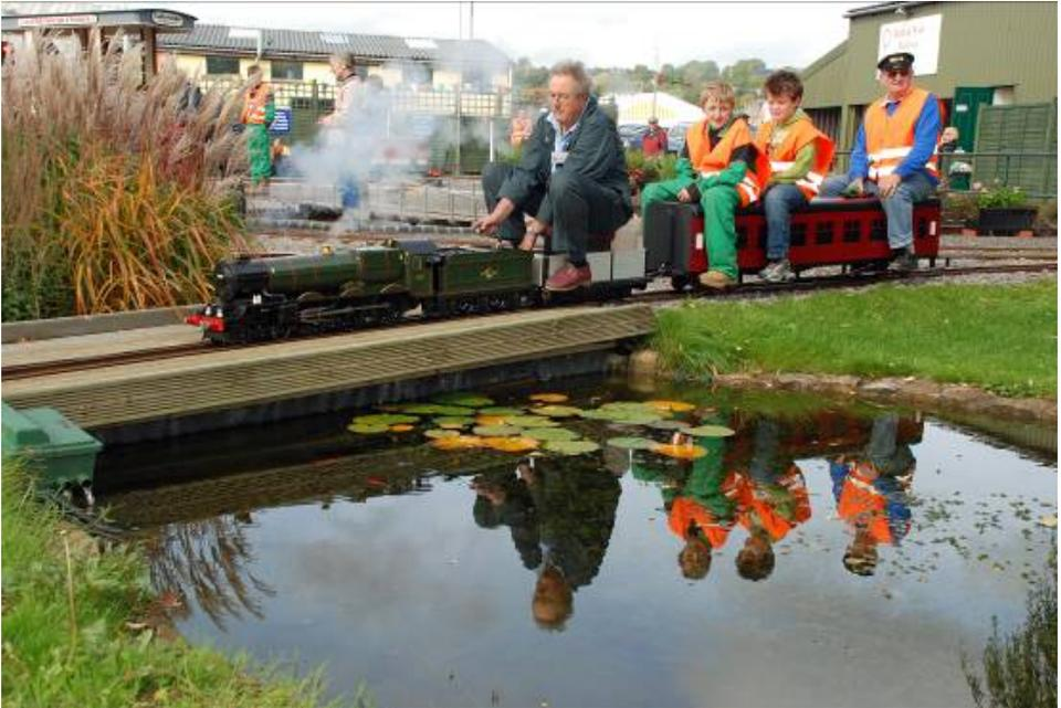
This view reveals that the railway benefits from attractive landscaping. A fine 5" gauge GWR 'King' crosses a bridge across a small pond on its way to distant parts. The carriage is of simple box construction with laser cut panels to simulate a railway-like appearance.
