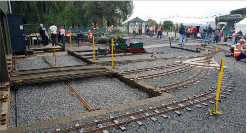
East Somerset SMEE. This view reveals a linear traverser, a 'bendy' rail section to four lines and a pivoting rail connecting three lines to the traverser.
